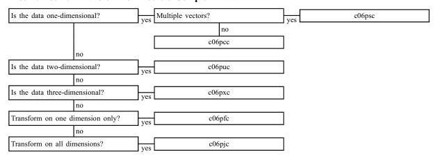
Tree 2: Fourier Transform of Real Data or Data in Complex Hermitian Form Resulting from the Transform of Real Data
