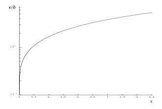
It should be noted that, for absolutely small x, the amplification factor tends to zero and eventually the error in the result will be limited by **machine precision**.
